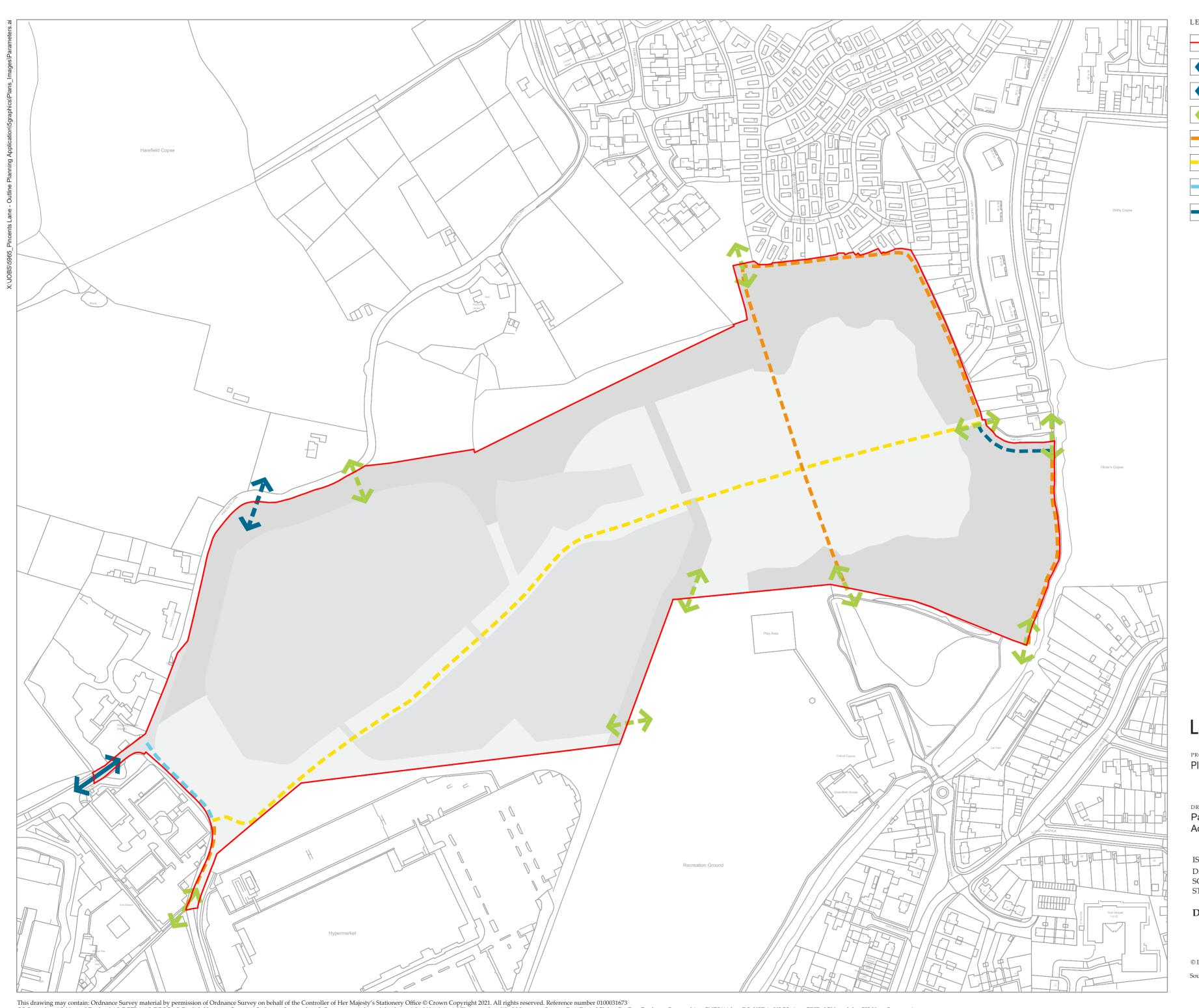
LEGEND Application boundary Vehicular access point Emergency vehicular access point Pedestrian access point Retained Public Right of Way Cycle path / retained Public Right of Way (separate paths) Shared cycle path and footpath Cycle path
